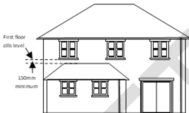
Figure 4.7: Single-storey extension with 150mm gap between extension ridge and windowsills of the first-floor windows.
